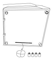
Screw feet into the corresponding pre-drilled holes by either rotating clockwise or using the provided hardware and tools. If your product has multiple feet types, additional detailed instructions will be included.
