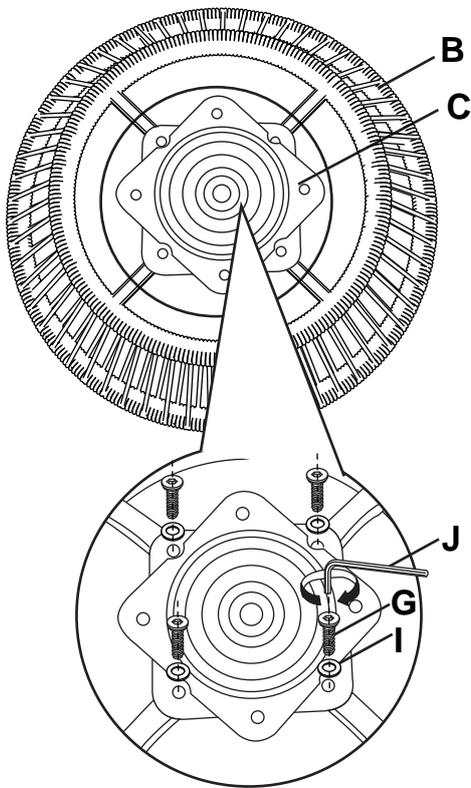
**2** Turn upside down seat top (A) on a protected surface, use Allen key (J) to fix seat base (B) on seat top (A) with bolts (G) and washers (I) as picture.
